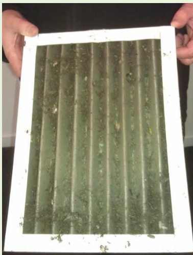
Figure 12: Insects blocking the MVHR filter
